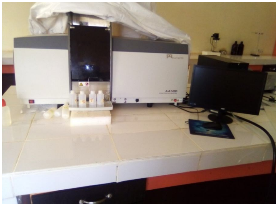
Figure 2. An atomic absorption spectrophotometer instrument in the laboratory.
